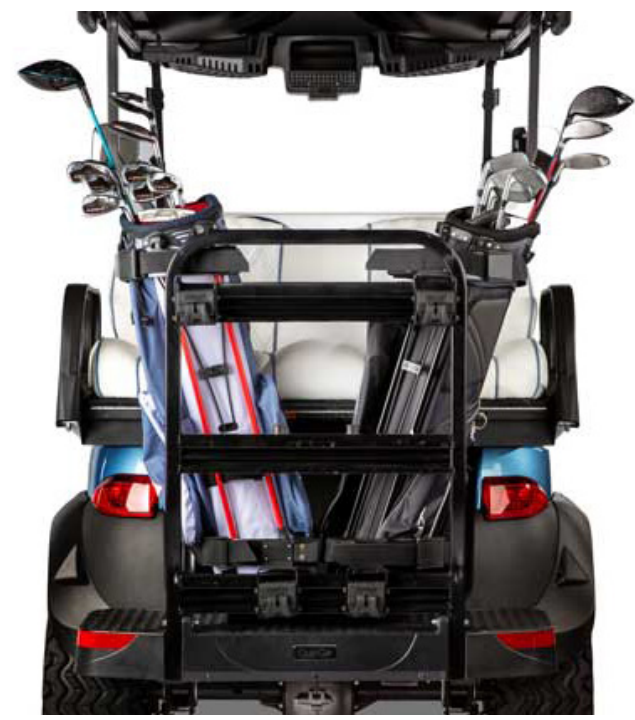
Innovative bag holder design angles the bags outward for easy access
